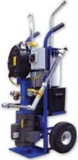
Our filter carts feature unique DFE rated filter elements to condition hydraulic fluids with double filtration with each pass through the filter cart. A wide range of media options are available with stainless wire mesh from 146 $\mu$  to .5 $\mu$ , water removal media, and varnish removal media. With flow rates of 5GPM, 10 GPM, and 22GPM and a wide variety of power options, these filter are carts ideal solutions for hydraulic fluid conditioning and cleaning oils during fluid transfer.
