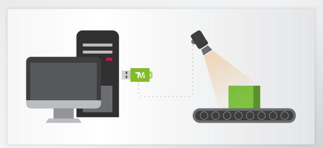
lines. After connecting the computer to external camera, the user can perform vision tasks like item recognition, image enhancement and measurement through TMvision™.
